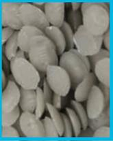
To create **3D models hollow inside**, should use a wax with particular characteristics: **soluble in water**.
