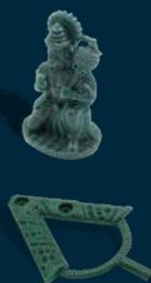
A wax with very low shrinkage and with higher viscosity than others, allows to obtain massive objects with well-defined details and without air bubbles inside. Its formula allows it to work at low temperatures, decreasing the cooling times of the mold.
